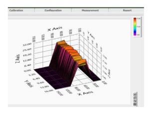
Fig. 9. 3D image of the analyzed belt fragment having width of 400 mm and mean thickness of 24.36 mm.
